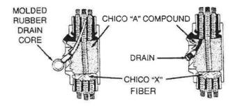
Remove large cover and pipe plug and dam the lower hub opening. Replace large cover threading as far as possible into body with arrow pointing directly down. Insert the molded rubber drain core through hole in large cover high enough so inner end will be above sealing compound in completed seal.
